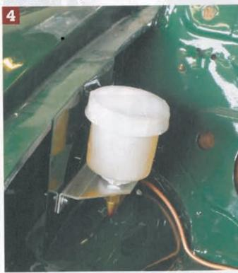
, whereas with the remote reservoir the fluid level can be checked from under the bonnet at a glance - a legal requirement in Germany where this Traveller was destined. Fitting is simple: the plastic reservoir is mounted under the bonnet and the feed pipe runs down inside the car ...
