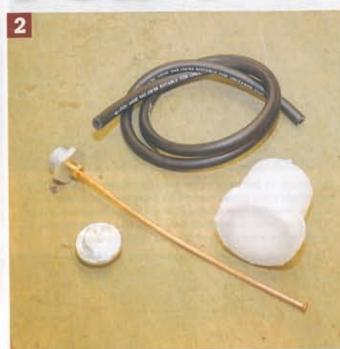
When converting from drums to discs, it's recommended that you install a remote fluid reservoir. The reason is that in a drum brake setup, the wear in the shoes is taken up by the manual adjustment you need to do in order to kep the brakes working properly. Disc brakes on the other hand don't have this adjustment so as the pads wear the calliper piston has to move further out and there's a danger of running too low on fluid with only the standard master cylinder.
