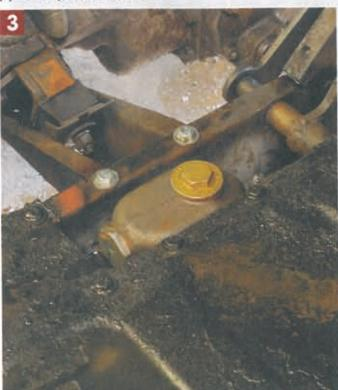
The remote reservoir can be fitted entirely separately from the rest of the brake upgrades and is worth doing as the standard Minor master cylinder lives in the chassis leg under the carpet. It's all too easy for the fluid level to get overlooked ...
