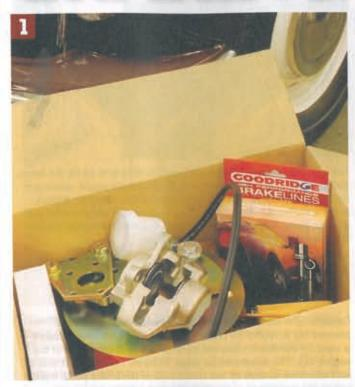
This is what you'll get if you order the full disc brake conversion: a pair of discs, a pair of brake callipers, the mounting brackets, backplates, the replacement hubs and a remote top-up reservoir. Plus of course all the crucial fitting brackets, bolts and brake pipes, ready cut and flared.
