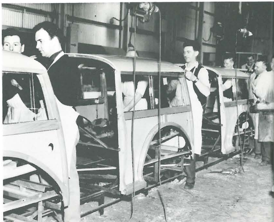
Skilled men assembling the aluminium and ash wood frame of the Traveller 1957.
