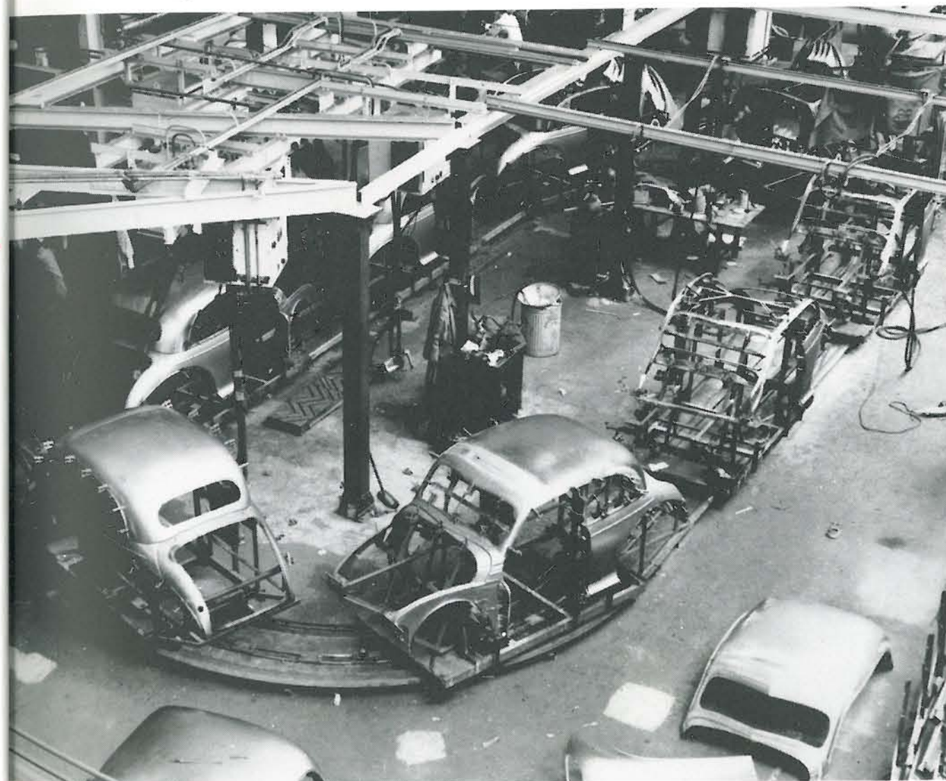
The body assembly line in 1949 showing how the different parts of the bodyshell are put together.
